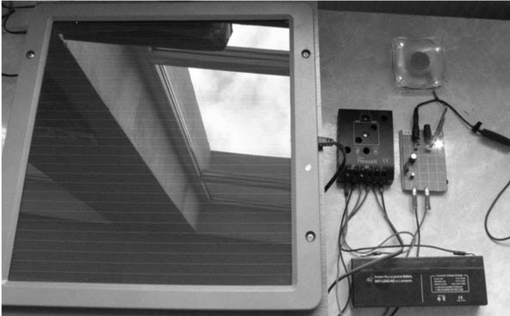
Fig. 6. Solar system consists of solar panel, controller, battery and consumer
